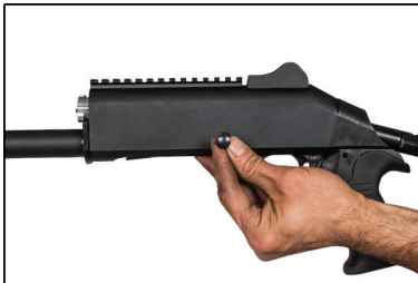
6) Take out the trigger group anchor pin.
