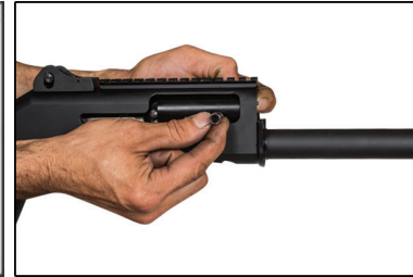
5) Move back the mechanism and ensure that cocking lever comes to the middle of the mechanism bearing; then, pull out and remove the cocking lever. During this operation,hold the cocking-bar so that the spring doesn't push it forward
