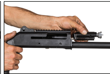
8) After you remove the Trigger Group, the bolt assembly and action bar sleeve can be removed from the shotgun
