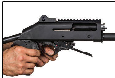
7) Pull the trigger group and detach from the receiver
